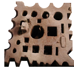
Swage anvil (also called a swage block)
